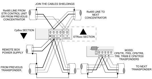
NOTE: +12V DOES NOT BELONG TO THE PREVIOUS DEVICE. THE IMAGE IS AN EXAMPLE OF REMOTE BOX POWER SUPPLY JOIN THE CABLES SHIELDINGS
