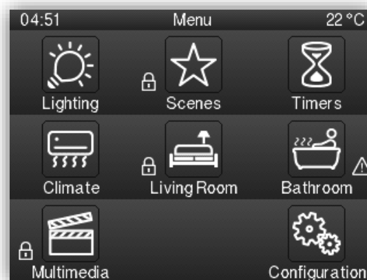
Figure 22. Menu with protection and alarms.
